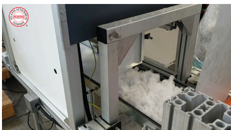
Shredder with infeed 500mm wide, equipped with bypass and external collecting silo Trituradora con entrada de 500 mm de ancho, equipada con by-pass y silo colector externo
