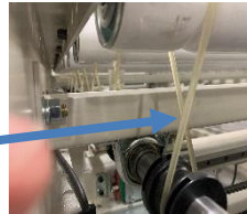
6. b. Check, align and clean conveyor belts and chain. Lubricate chain, bearings.
