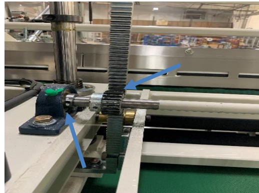
6. b. Check, align and clean conveyor belts and chain. Lubricate chain, bearings.
