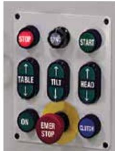
Convenient front mounted controls. Power table and power tilt. Micro speed adjustment for sewing head allows perfect synchronization with carriage.
