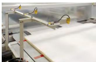
Unique “no contact” photocell arrays adjust side seals without distorting stack.
