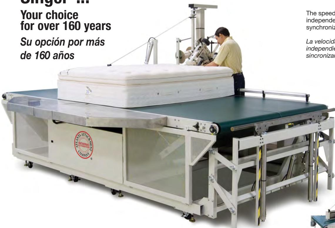
The speed of the sewing head can be independently adjusted by the operator for synchronizing head and belt (no more tugging).
