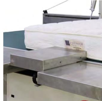
After flip, mattress is automatically relocated to the sewing head. No tugging by the operator.
