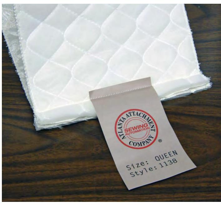
Inserts a control label on top of the seam. Label is hidden from view, inside mattress.
