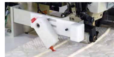
**3200PM option** Automatic Marking Module Marks border for placement of handles
