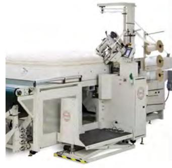
Operator platform automatically raises and lowers with sewing head to maintain operator's ergonomically correct height.
