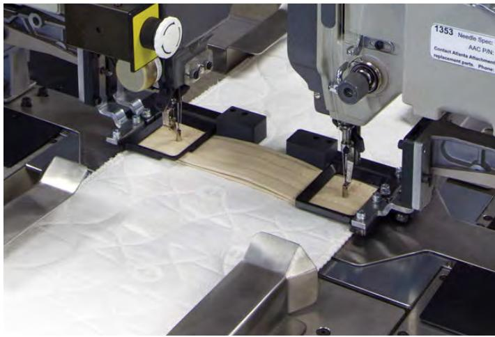
Vertical handle, heads positioned side-by-side.
