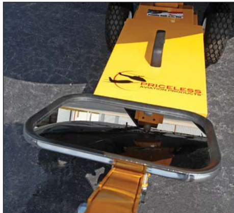
Robinson Ball Hitch shown in mirror from perspective of user
