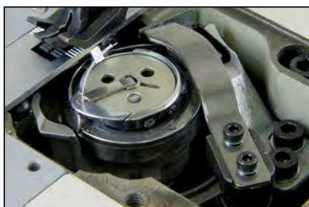
Automatic thread trimming device. Large bobbin capacity.
