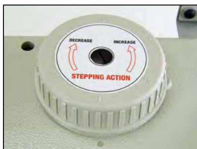
Top dial for convenient adjustment of walking feet for different material thicknesses.
