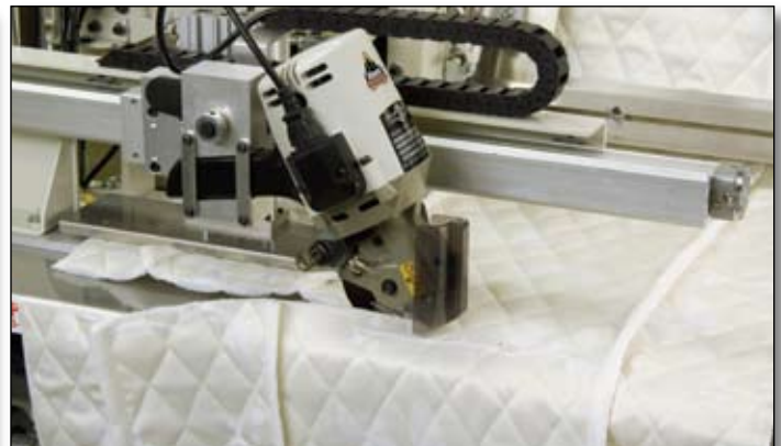
Optional semi-automatic cutter available, replaces marker
