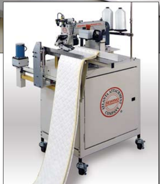
Top belt feed swings out for threading and other maintenance
