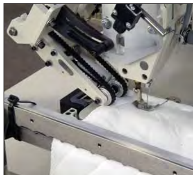
Top belt feed swings out for threading and other maintenance
