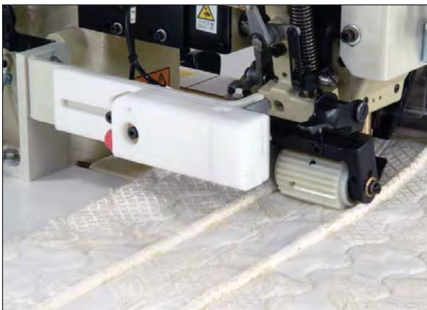
Automatic Marking Module - Marks border for placement of handles - Model 3200PM
