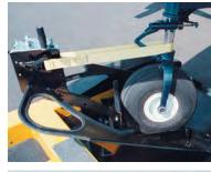
Wench with durable webbing rotates with Lazy-Susan™ turntable insuring no stress is placed on the nose gear.
