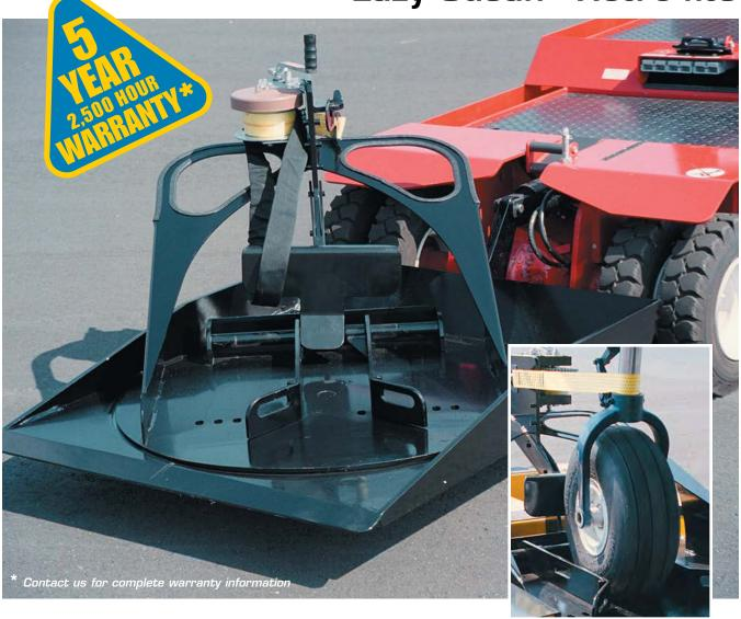
Priceless Plane Products<sup>™</sup> offers a Lazy Susan<sup>™</sup> retrofit bucket for all models of JetPorter and Lektro tugs. This turn-table allows 360 degree rotation. Linemen can turn with no restrictions and since the turn-limit of the aircraft cannot be exceeded, risk of damage to the nose gear is eliminated.
