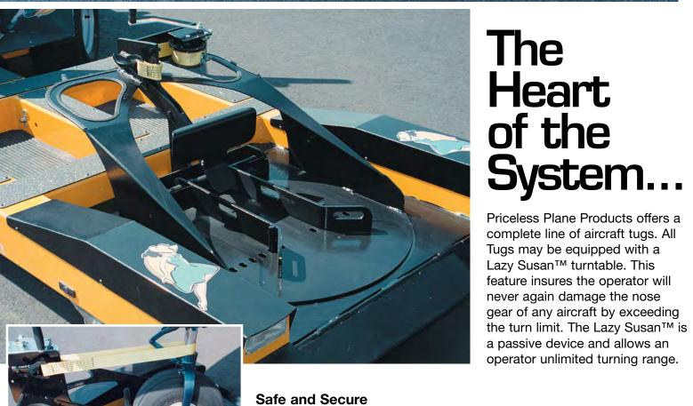
With the aircraft"s nose gear seated and secured into the Lazy Susan, handlers are assured of unequaled mobility with no danger of damaging the gear.
