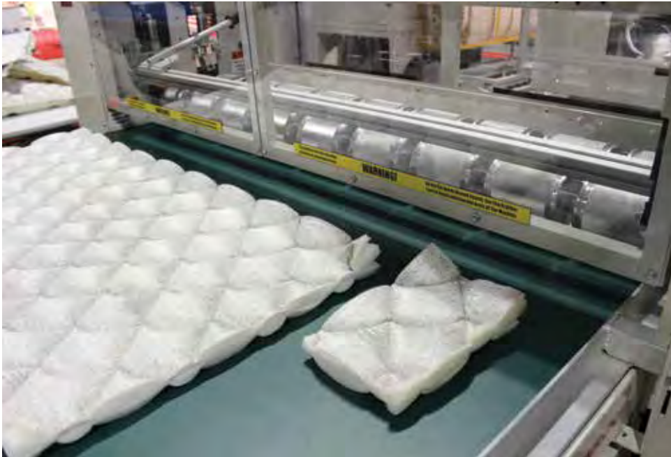
The small peice of panel shown for use on mattress edge support.
