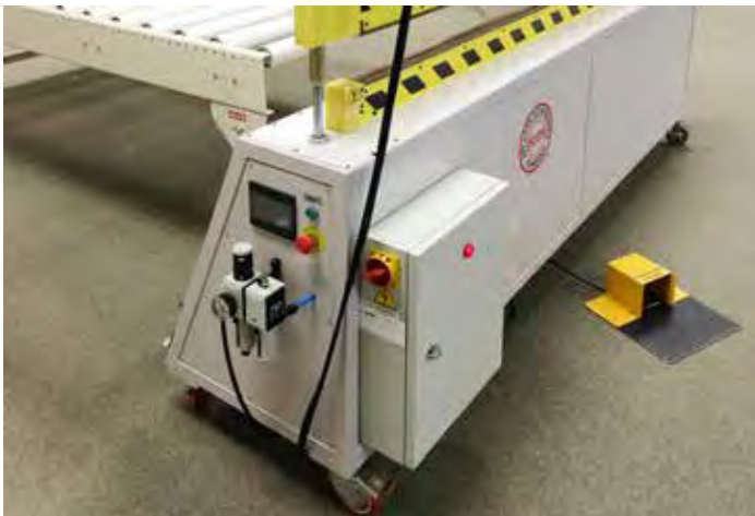
PLC Controls / Controles PLC
